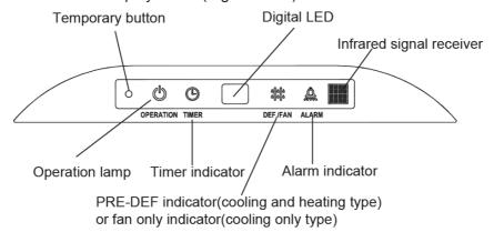
2.1.2 Icon explanation on indoor display board (Compact cassette & High static pressure Duct).
